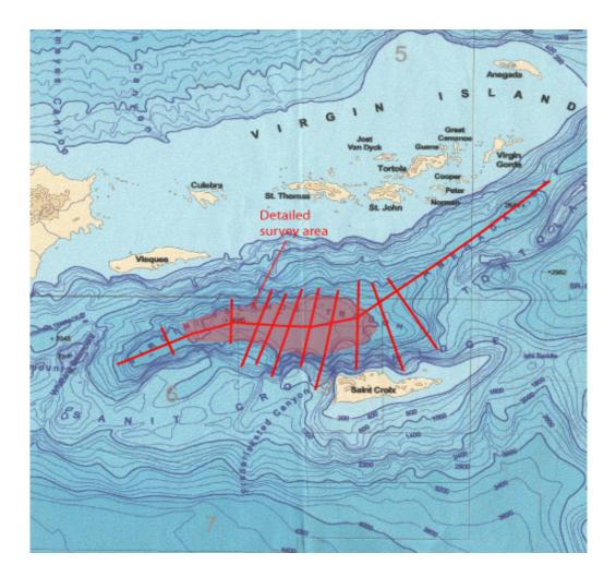
**Fig. 1** Bathymetry of Caribbean waters around the former Danish West Indies with a tentative multi-channel seismic grid (red lines) and detailed survey area (ligh red) in the southern part of the Anegada-Jungfern Passage .
