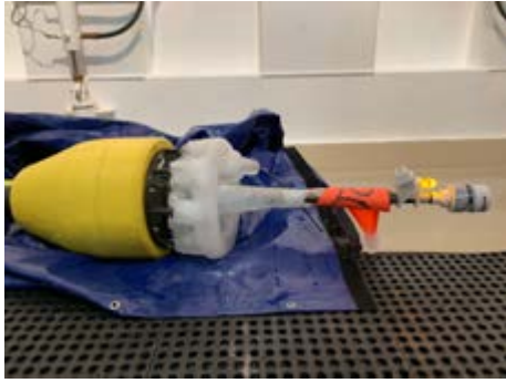
Figure 5.9: SWIFT20 upon recovery from the open ocean deployment. All location devices were covered by ice.
