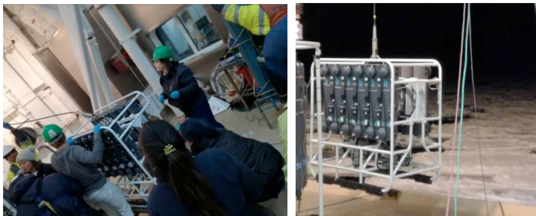
Figure 15.3. Preparation (left panel) and deployment (right panel) of "mini-GoFlo" rosette for trace metal clean sampling in the marginal ice zone.
