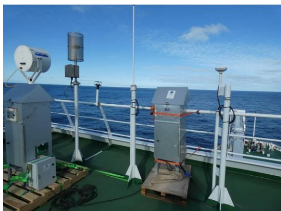
Figure 15.1. High-Volume air sampler on Monkey Island (SA Agulhas II). The TRACEX dust sampler was connected to a wind-direction control switch from the Team NAIR.
