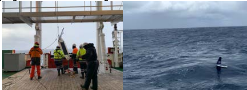
Figure 5.8: Deployment of the Sailbuoy using the bow ring (left) and post deployment, sailing away from the ship (right)
