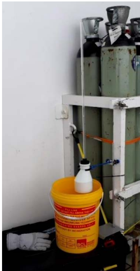
Figure 13.27 Schematic of the Falling Head Permeability Test [Kuroiwa 1967] and the permeability testing prototype used on the ship.
