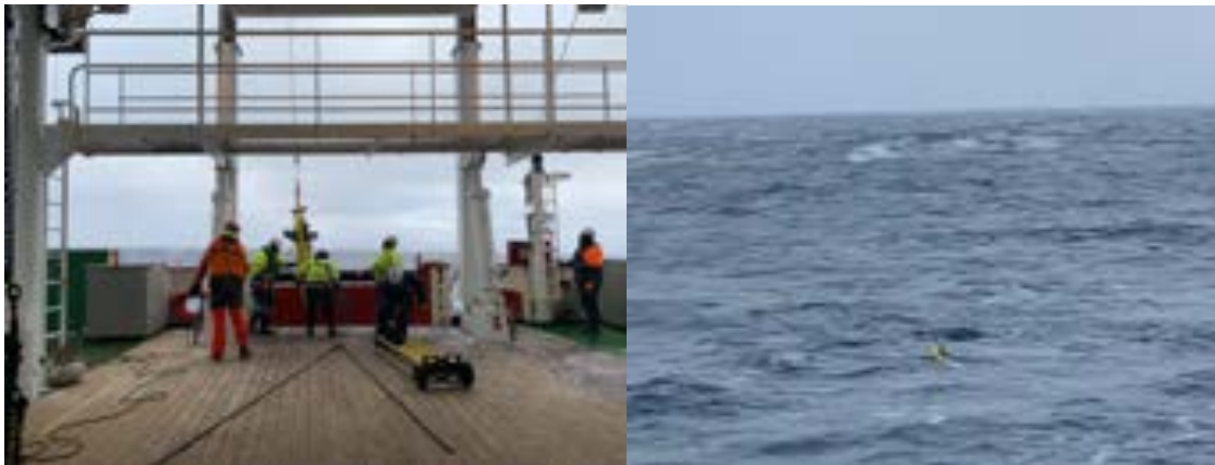
Figure 5.7: Deployment of SG662 (left), and the buoyancy position in the water after 5 minutes (right)
