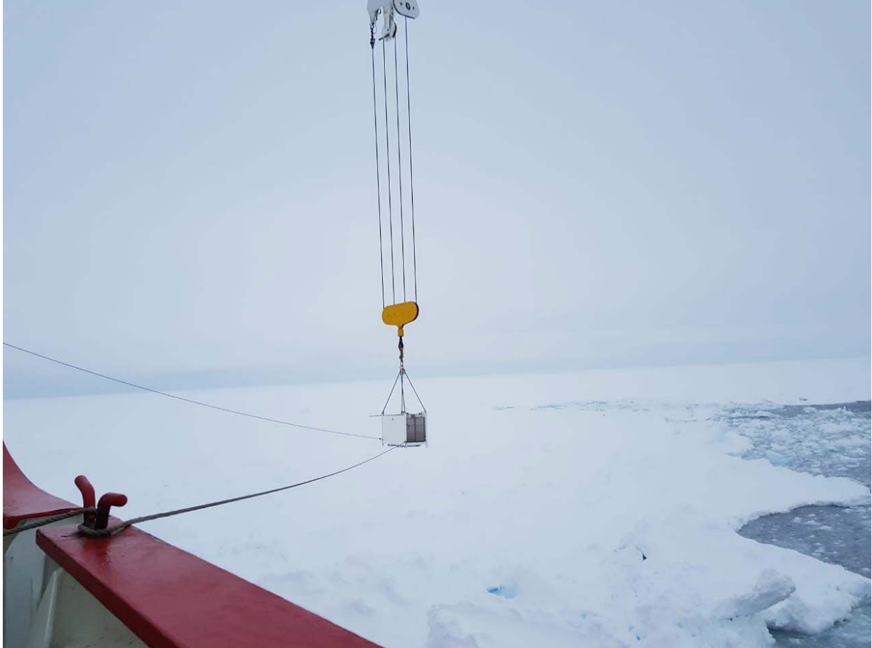
Figure 4.5: Instruments were cable tied to poles across the gondola and then lowered by crane.
