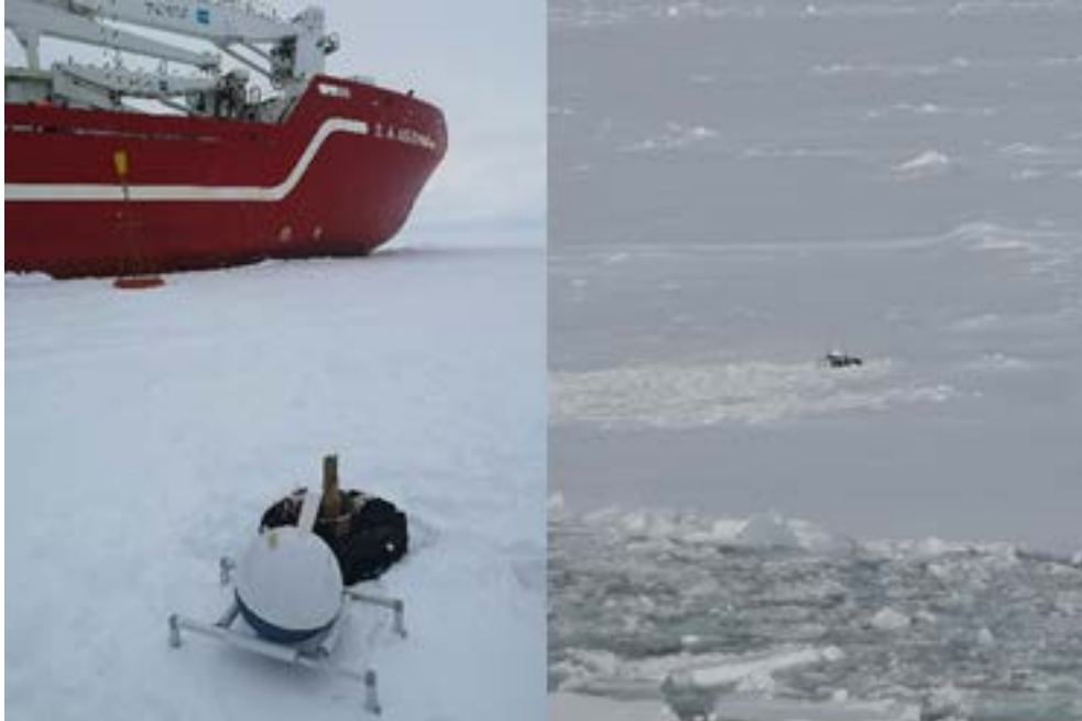
Figure 12.9. Deployment of a standard iSVP buoy on specially-designed cradle, on a floe in the MIZ.
