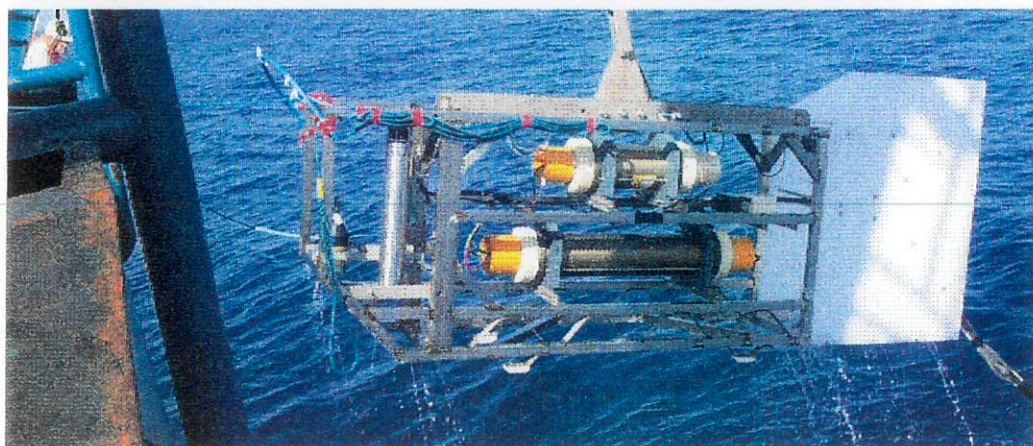
Figure 7. The DASI deep-towed transmitter system during deployment and recovery. The neutrally buoyant antenna streamer can be seen trailing just below the surface in the upper two pictures.
