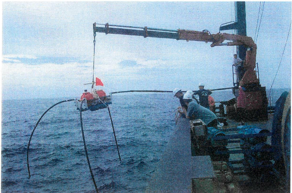
Figure 9. Deploying a LEMUR. The two orange plastic casings contain glass spheres. That on the left houses the recording electronics and acoustic release; while that on the right is for buoyancy only. The electrodes are housed in the ends of the flexible black arms. The black cylinder on top of the left hand sphere is the acoustic transducer. The bottom weight (coloured blue and green) can be seen underneath the instrument frame.
