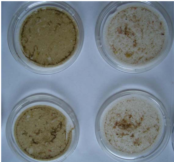
Figure 7.15.2: GFF filters for analysis - P1 (Left 1/40th splits from 150m) and P2 (Right 1/32nd splits from 250m)
