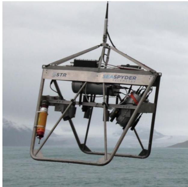
Figure 2. Deployment of the drop camera frame from the aft starboard crane of the RRS Discovery
