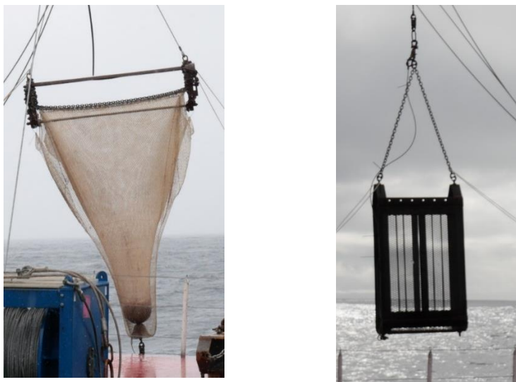
Figure 3. Recovery of the Agassiz trawl (left) and dredge (right) from the aft deck of the RSS Discovery during cruise code DY099 showing the bridles, weak links and recovery bridle (dredge).
