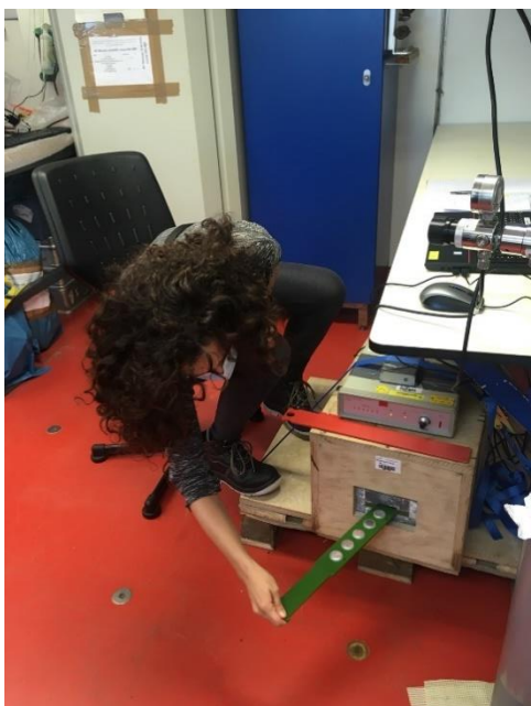
Fig. 12.4 Measurements of dissolve or particulate \text{Th}_{234} on the Risø low-level beta GM multicounter.
