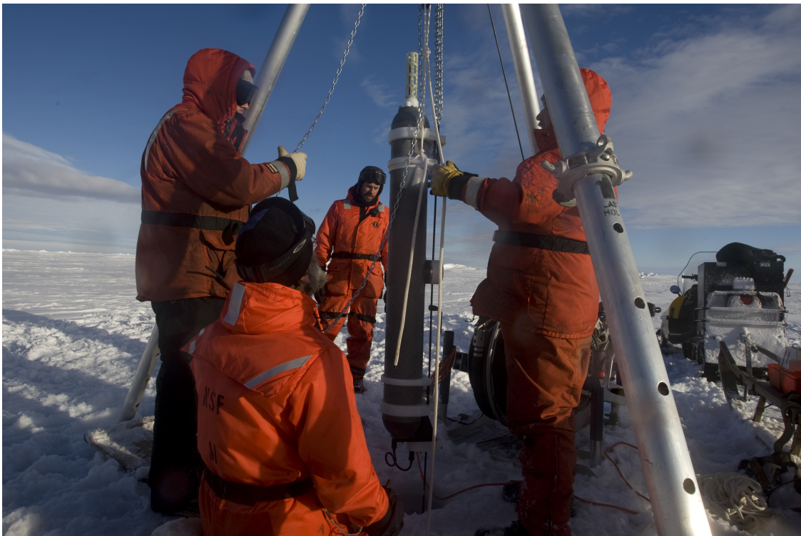
Figure 23: ITP mooring deployment photo showing tripod, ITP, and ice hole. Image © Maria Stenzel, 2009
