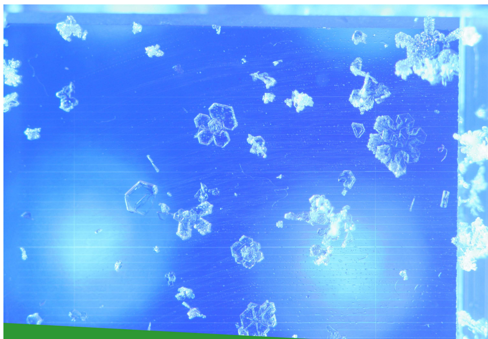
Figure 44: Snow captured during the February 4-5 event while the NBP was conducting a ctd transect along the Dotson Ice Shelf. The white lines are 200 \mu\text{m} (0.0002 m) apart.
